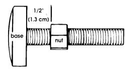
Use legs and nuts from parts package. Screw nut down to within 1/2 inch (1.3 cm) of base.
